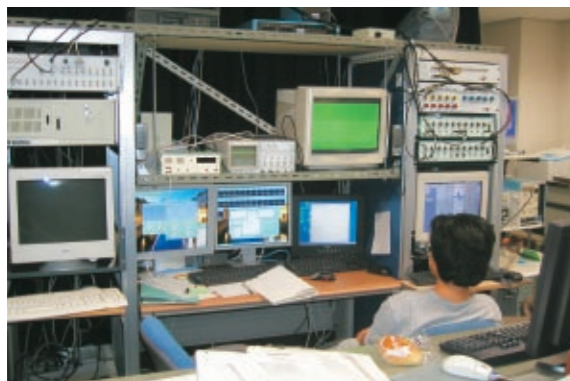
視覚神経系研究のための実験システム Data acquisition and experiment control system for studying responses of visual neurons.
