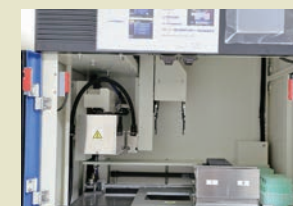
DNA自動分離装置 Automatic plasmid DNA preparation device: Gene Prep Srar PI-480
