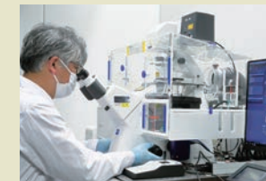
超解像共焦点顕微鏡 Super-resolution confocal microscope: LSM 900 with Airyscan 2
